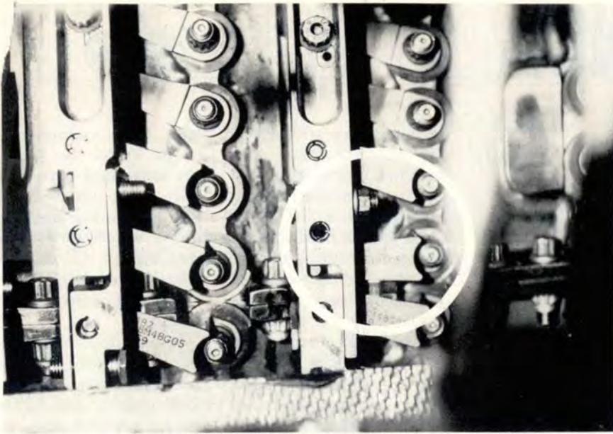
This lever arm pin is trapped between the actuation rings and not inside the pinhole.
